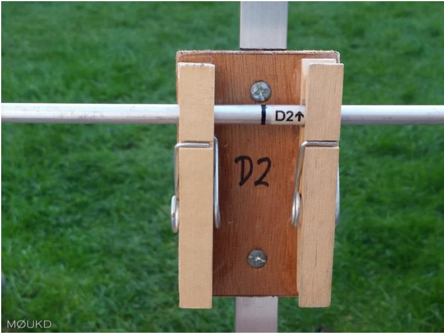
An element in place. The black line is centred to the screw, which is centred to the boom.
