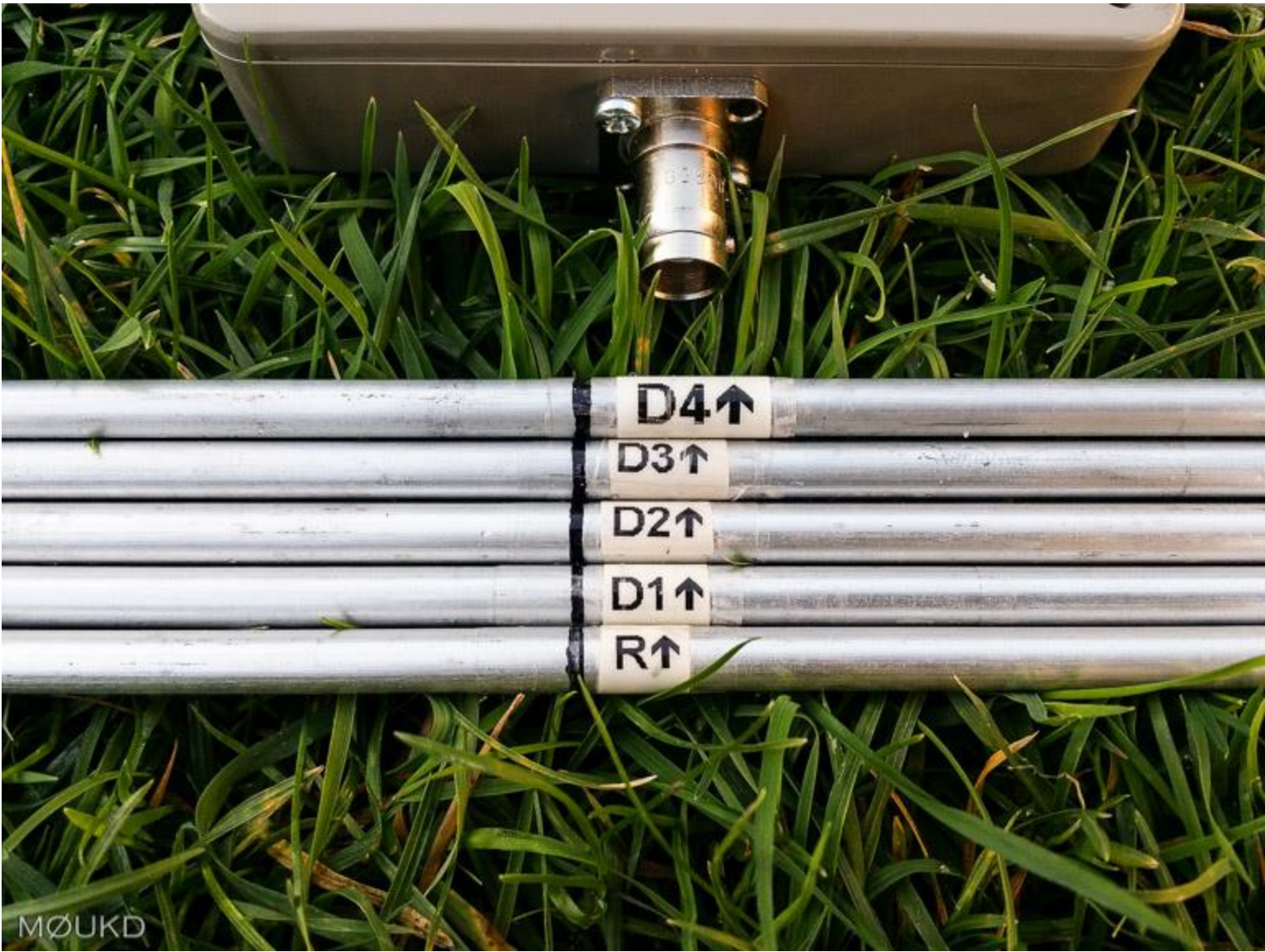
The elements are numbered and marked with a black centre line for ease of assembly.
